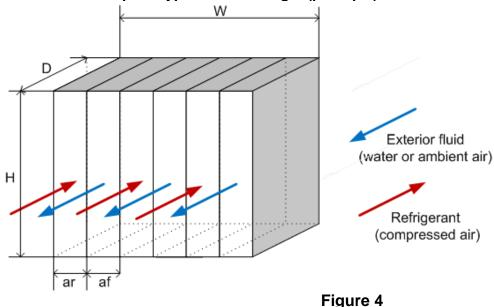
This type of exchanger is not used in this paper, but cross-flow exchangers are calculated as counter-flow exchangers, with a reduction of efficiency for the air-air exchanger.
