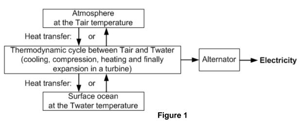
As shown in the figure 1, the plant can work in two configurations:
